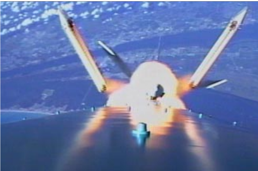
The Florida coastline is visible below this Delta II rocket as its solid-fuel boosters fall away while the launch vehicle continues on. This photo, taken from a Boeing video, depicts the launch of NASA's Mars Odyssey payload.
