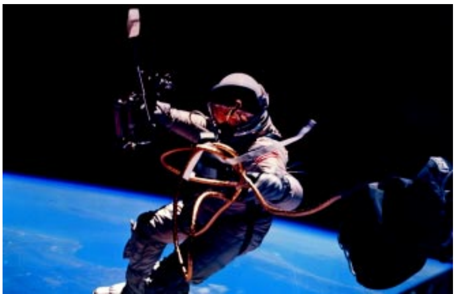
Astronaut and USAF Maj. Edward White II became the first American to walk in space during the Gemini 4 mission on June 4, 1965. White was attached to the spacecraft by a 25-foot umbilical line and a 23-foot tether line, both wrapped in gold tape to form one cord.
